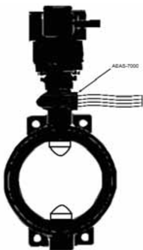
Figure 3. Diagram displaying mounting of Avago's absolute encoder on a butterfly valve
